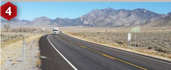
**Constraint:** Throughout the US 93 Corridor there are very few turn lanes for acceleration and deceleration at cross streets in the high-speed areas which causes delays at locations with high turn volumes, and contributes to rear-end crashes in high-speed locations
